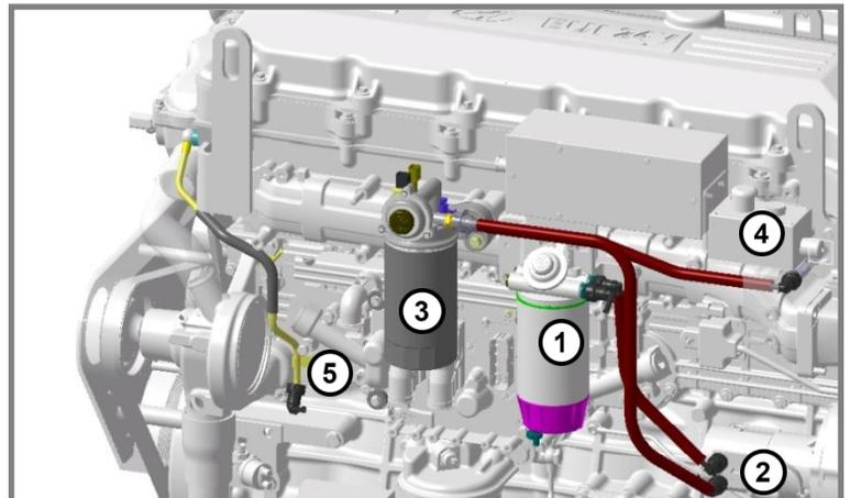
※ The minimum inner diameter of the fuel hoses should be at least  $\varnothing 10$
