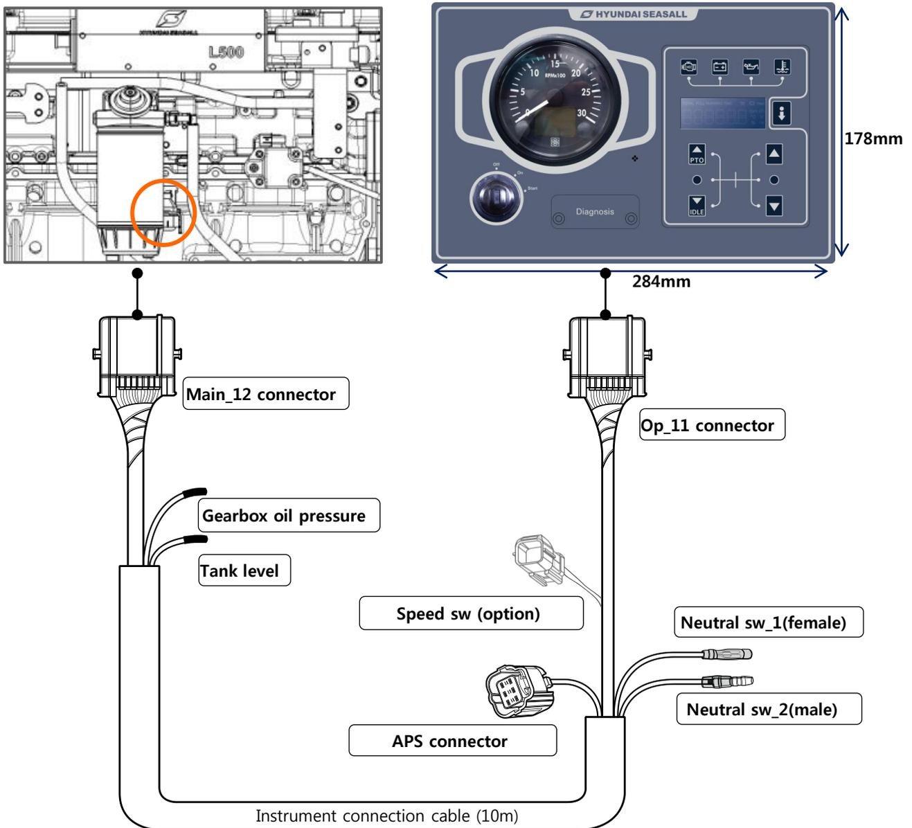
※ If there is no neutral switch, you must connect the neutral switch-1 and neutral switch-2 of the instrument connection cable.
